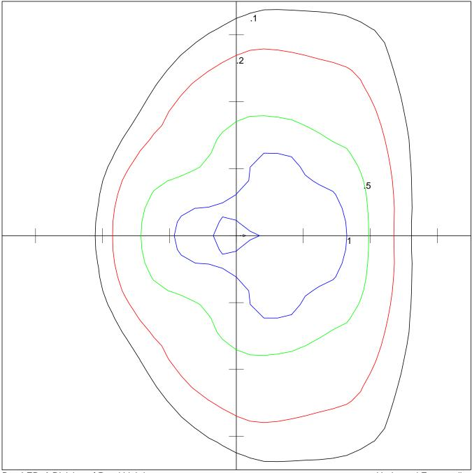
BetaLED, A Division of Ruud Lighting ARE-EDG-3M-\*\*-12-C-27 (350mA) SCALED FROM 120 LED TYPE III MEDIUM EDGE 350mA SCALED FROM ONE HUNDRED TWENTY WHITE LIGHT EMITTING DIODES (LEDS), Horizontal Footcandles
