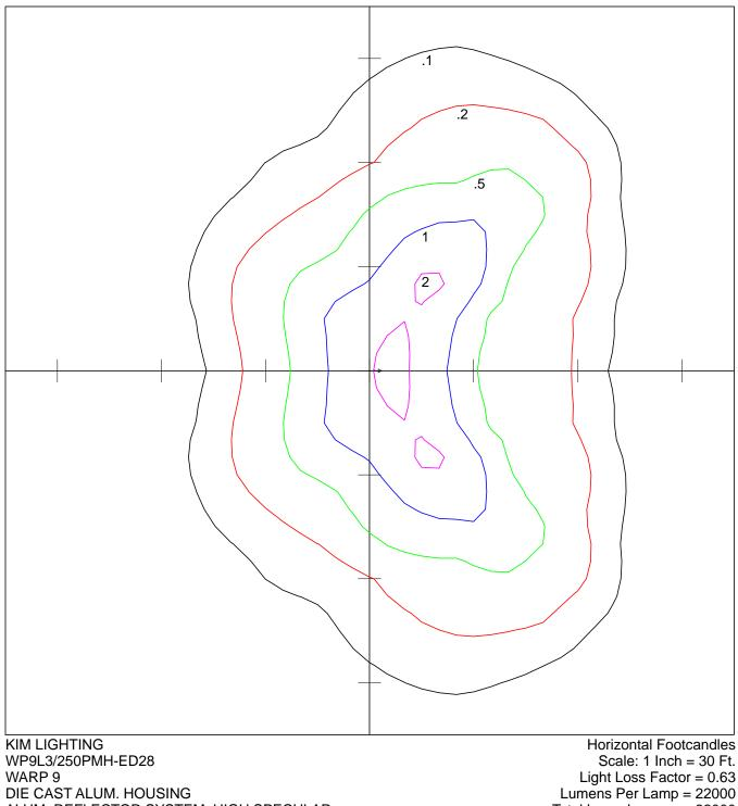
DIE CAST ALUM. HOUSING ALUM. REFLECTOR SYSTEM, HIGH SPECULAR REFLECTIVE PANELS CLEAR FLAT GLASS LENS 250 WATT PMH CLEAR ED-28 MOGUL BASE Horizontal Footcandles Scale: 1 Inch = 30 Ft. Light Loss Factor = 0.63 Lumens Per Lamp = 22000 Total Lamp Lumens = 22000 Mounting Height = 25.00 Ft Maximum Calculated Value = 2.19 Fc Arrangement: Single Arm Length = 1.5 Ft
